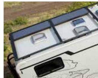
Solar power system
